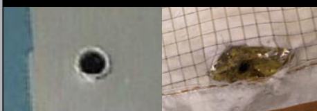
A 1.4mm diameter (inside) hole found March 2001 in an ISS mini-pressurized logistics module outer bumper panel (no damage reported to pressure shell). This 6cm (2.4in) x 3cm (1.2in) hole in the thermal blanket over the MMOD shield was found by crew in June 2007.
