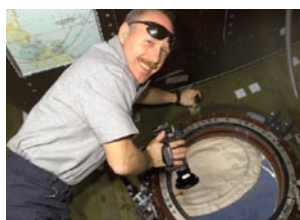
US Lab in orbit, above Ken Bowersox uses camera at window with partially deployed shutter; to right window shutter fully deployed; outer debris shields are visible.
