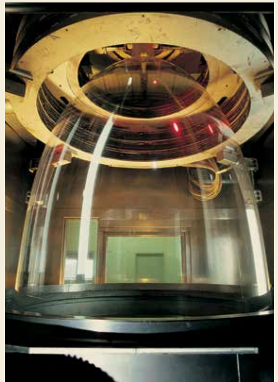
The unique 'bubble' process used to manufacture Clarity®C film
